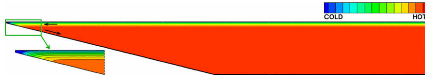
Fig. 4. Isotherms at the initial stage of the flow development (conductive effect, Gr = 10^7 , Pr = 7.01 , and t = 120 s). The dark arrows represent the direction of the convective circulation.
